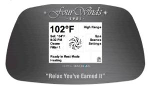
Ready-in-Rest Mode appears if the spa is in Rest Mode and Pump 1 is activated. When the heater pump comes on automatically (ex: for heating) you can switch between low and high speed but cannot turn the heater pump off. After 1 hour, system reverts to Rest Mode.
